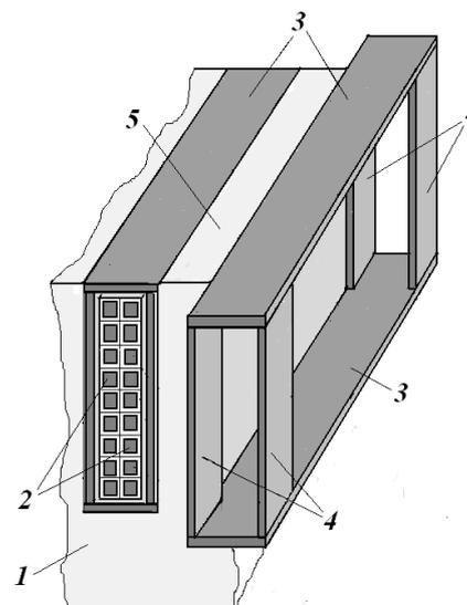
Figure 3. Using of the Shield 2 in the model (1 is the ferromagnetic core, 2 are sections of winding, 3 are the copper plates, 4 are the conducting brattices). The brattices at the left side of pictures are omitted
