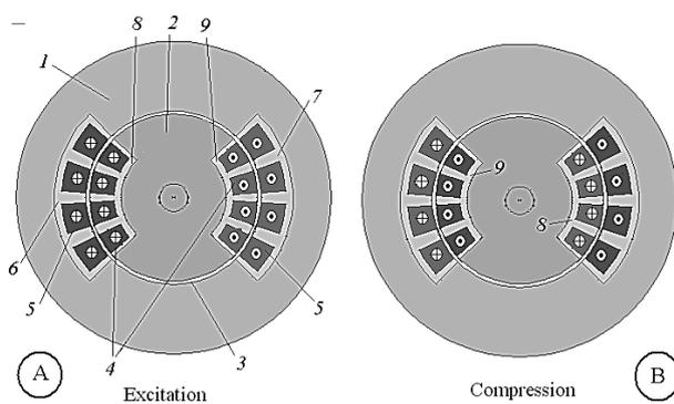
**Figure 8. The cross section of the compression generator at two positions of rotor: A – for the excitation of the initial magnetic field, B – for the stage of the flux compression. Designations: 1 is the stator core, 2 is the rotor core, 3 is the air gap, 4 is the rotor winding, 5 is the stator winding, 6 and 7 are the block-keepers of stator winding, 8 and 9 are the block-keepers of rotor winding**
