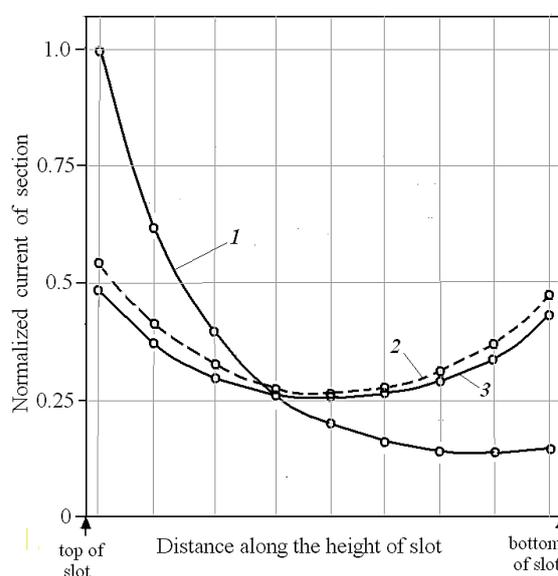
**Figure 7. Distribution of current in the sections of winding at the frequency 400 Hz (1 is the mode of compression; 2 are the inner sections, mode of excitation; 3 are outer sections, mode of excitation). The basic current is equal to 1 A**
