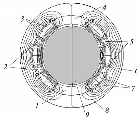
**Figure 9. Cross section of magnetic system of generator with a picture of the field lines in the stage of the flux compression. Designations: 1 and 4 are the big teeth (poles) of stator core; 2 and 5 are the small teeth of stator; 3 and 7 are the winding conductors; 6 is the flux lines in the yoke; 8 is a yoke of stator; 9 is a rotor of generator. Details of rotor design are omitted**
