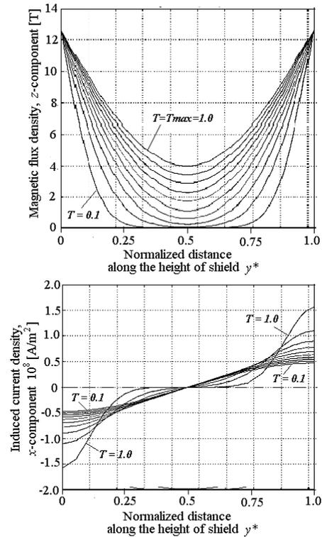
**Figure 11. Results of simulation for the flux switch in across the conducting plate likely to Shield 1**
