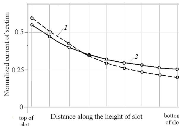
**Figure 6. Distribution of current in the section of winding at the frequency 50 Hz (1 is the mode of compression; 2 is the mode of excitation at coupling connection of both windings). The basic value of current is equal to 1 A**
