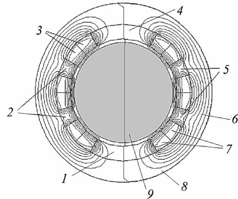
**Figure 9. Cross section of magnetic system of generator with a picture of the field lines in the stage of the flux compression. Designations: 1 and 4 are the big teeth (poles) of stator core; 2 and 5 are the small teeth of stator; 3 and 7 are the winding conductors; 6 is the flux lines in the yoke; 8 is a yoke of stator; 9 is a rotor of generator. Details of rotor design are omitted**
