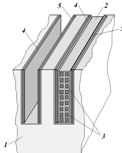
Figure 2. Using of the Shield 1 in the model (1 is the ferromagnetic core, 2 is the winding package, 3 is the sections of winding, 4 is the copper plate at left side of slot, 5 is the copper plate at the right side of slot)
