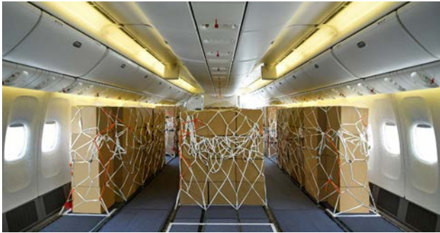
Fig. 3. Air Canada passenger Boeing 777 convertible for cargo on the upper deck due to declining demand for passenger traffic during the COVID-19 pandemic
