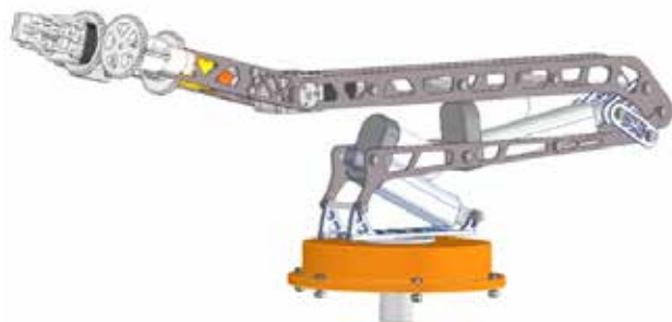
Fig. 20. Manipulator after optimization of links
