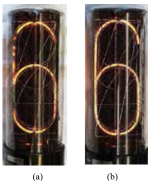
Fig. 6. Partially «poisoned» cathode (a), cathode of the indicator after recovery with increased current (b)
