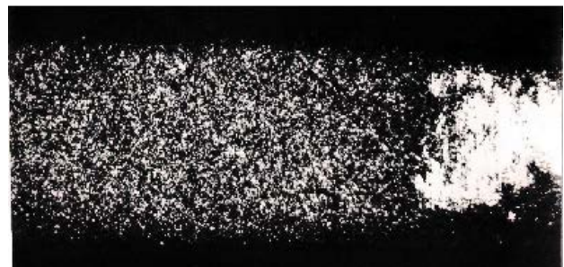
Fig. 1. View of the contact surface treated with waterjet
