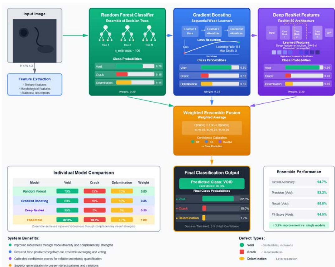
Fig. 3. Ensemble defect classification system combining Random Forest, Gradient Boosting, and deep ResNet features
